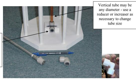
Connector must be installed at the base of the model. Use the 3/8" diameter connector as supplied by the Model Water Tower Competition.
